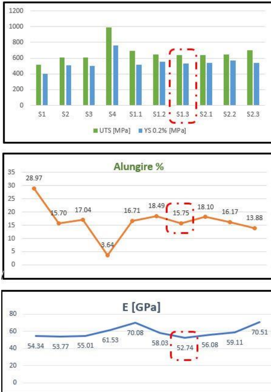
Figure 5. - Evolution of the mechanical properties for the studied alloy at all stages of the experimental program: (a) ultimate tensile strength [MPa] - Rm; yield strength [MPa] - (Rp0.2); (b) elongation at break (%) - \epsilon ; (c) modulus of elasticity [GPa] - E.
